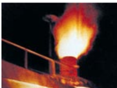
Soot fire raging from the stack.
