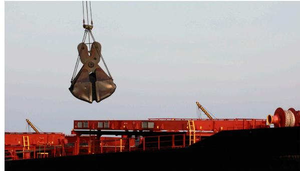
An AB was operating the crane for lifting the grabs. On the quay were two cadets, the third officer, two ABs and the vessel's superintendent. The chief officer had instructed the two cadets to only help if specifically needed. The ABs were instructed to remove the wires when the grab was safely secured on the trailer.
