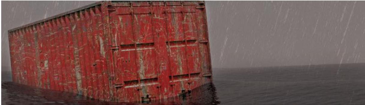
The large container vessel was sailing on a SE course in the North Atlantic, bound for a European port. During the voyage, heavy weather was encountered from ENE at Beaufort scale 9, with 7 m waves. This meant that the wind hit the vessel on its port side, causing heavy rolling. The maximum rolling was 20° to starboard and 30° to port.
