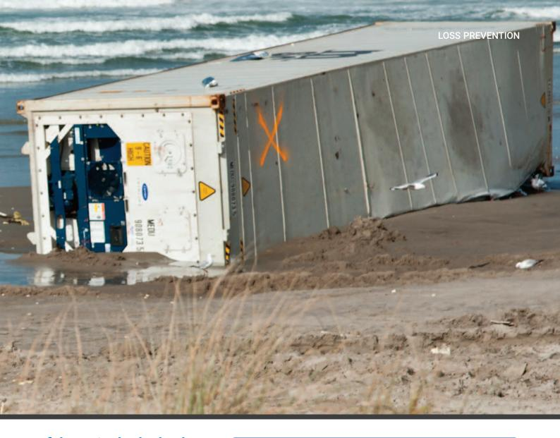
If the twist locks had been properly fastened they would have been damaged but would have remained attached to the toppled containers.
