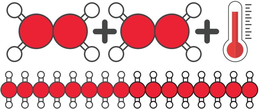
If the concentration of inhibitor or oxygen falls too far then the rate of polymerisation may increase to a point at which heat is produced very quickly and the temperature becomes very high.
