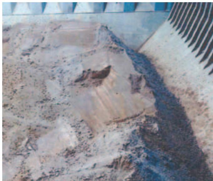
Photograph of iron ore fines showing spatter on the side of the hold caused during loading by excess moisture in the cargo.
