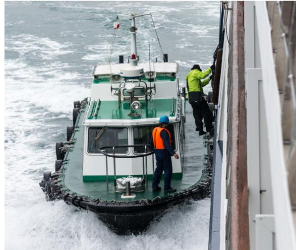
The plan was for the technicians to disembark from the bow of the tug. The first technician climbed up the ladder without any problems. There was a slight swell, so it was important to time the climb up correctly. The second technician grabbed the pilot ladder but at the same time a big wave hit the tug. This caused the technician to lose his balance and grip and he fell into the water.
