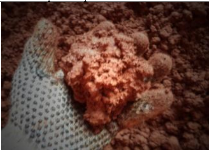
Bauxite cargo with signs of liquefaction
