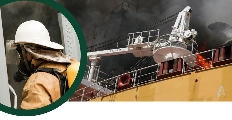
crew monitored the temperature of the engine room which was coming down. About an hour after the first CO<sub>2</sub> was released, smoke stopped coming out of the funnel.
