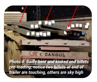
The bars must be handled at all times with a long spreader bar, preferably equipped with fabric slings, to avoid material droop. Severe damage can be caused by forklift handling where the billets overhang the forklift tines by any appreciable distance.
