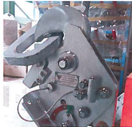
[Figure 4] Abnormal condition of link
