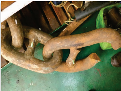
Photo 1: Failed common link to anchor chain resulting in loss of chain and anchor
