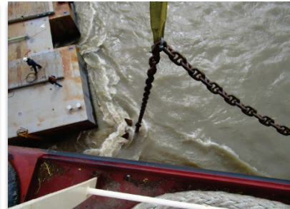
Photo 9: Floating crane barge assistance in recovering an anchor
