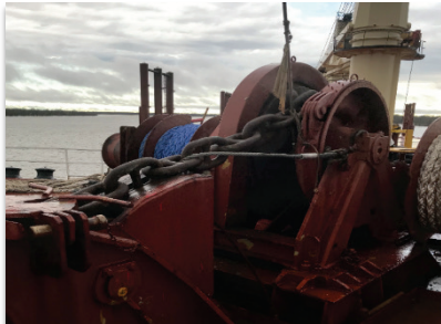
Photo 7: Proper securing of the anchor chain with disengagement of the gear reduces the risk of winch or motor damage
