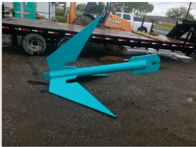
Photo 10: Typical grapple hook for attempted lost anchor recovery
