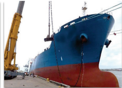
Photo 12: Fitting a new anchor and chain with mobile shore crane assistance
