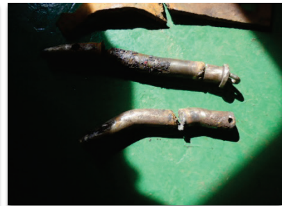
Photo 3: Failed stopper pins from the anchor windlass guillotine stopper
