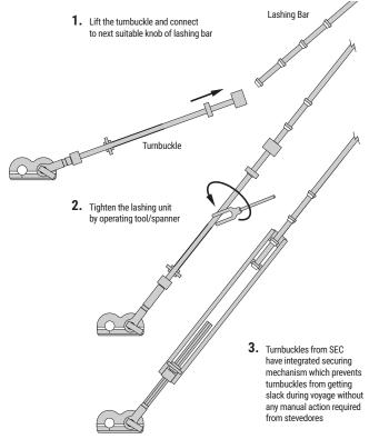
Correct securing of containers. Courtesy: SEC Bremen
