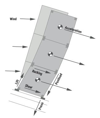
The mass of the containers will be accelerated by the movements of the ship as a response to the sea conditions. *Courtesy: Macgregor*
