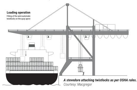
SATs lock automatically and require manually unlocking before unloading begins. FATs do not need any manual operation. All twistlocks have the same safe working load (SWL) of 25 tonnes but the more important figure is the pull-out force or holding power. This is tested by the classification societies. Heavy duty FATs can take higher loads, the safety factor between safe working load and minimum breaking load is four times instead of two times for a light FAT.
