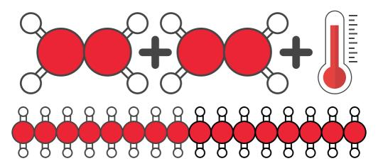
If the concentration of inhibitor or oxygen falls too far then the rate of polymerisation may increase to a point at which heat is produced very quickly and the temperature becomes very high.
