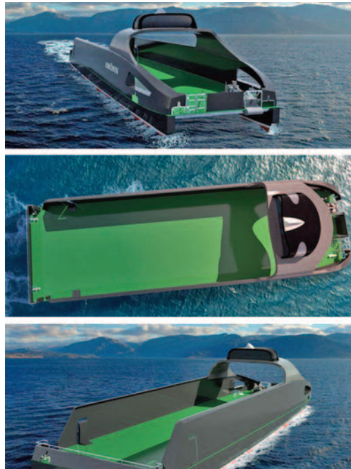
Hrönn, the world’s first unmanned and fully automated offshore vessel (Kongsberg Maritime)
