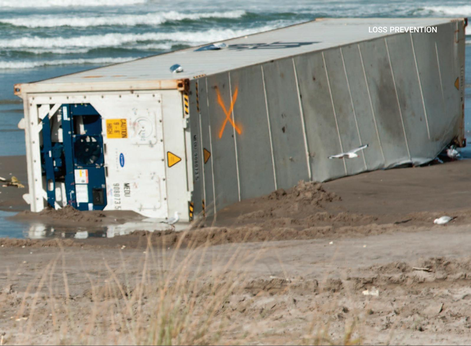
***If the twist locks had been properly fastened they would have been damaged but would have remained attached to the toppled containers.***
