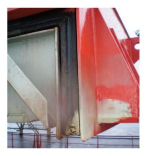
When replacing the gaskets the hatch cover bearing pads should also be checked or repaired as worn bearing pads can cause over-compression of the gaskets resulting in a shortened lifetime.
