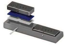
Hatch cover bearing pads transfer the weight of the cover, and any cargo it may be carrying, to the ship's hull while allowing for relative movement between the cover and the hatch coaming caused by hull flexing in a seaway. They must also maintain the correct compression on the hatch cover gasket and avoid wearing damage to the coaming/hatch cover interface.
